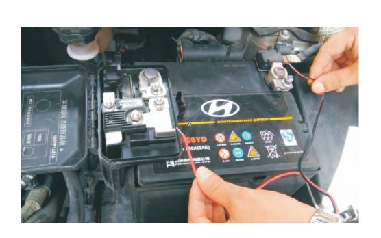
Simply connect the red and black wires to the positive and negative terminals of the car battery: red to the positive(+), black to the negative(-).
