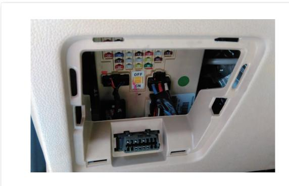
Locate the wire bank/ fuse box of the vehicle - it is typically in the front under or near the steering wheel - and connect the red and black wires there. Use the blue clips if needed.
